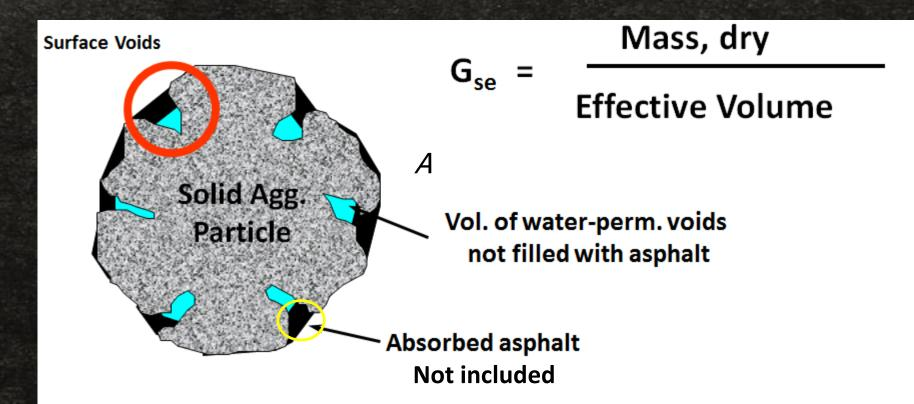
Effective volume = volume of solid aggregate particle + volume of surface voids not filled with asphalt
