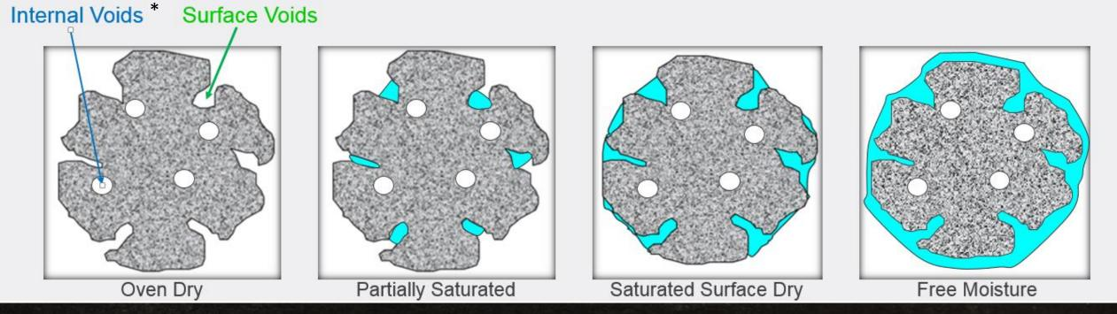
**\*NORMALLY INTERNAL VOIDS ARE NOT CONSIDERED IN AGGREGATES**
