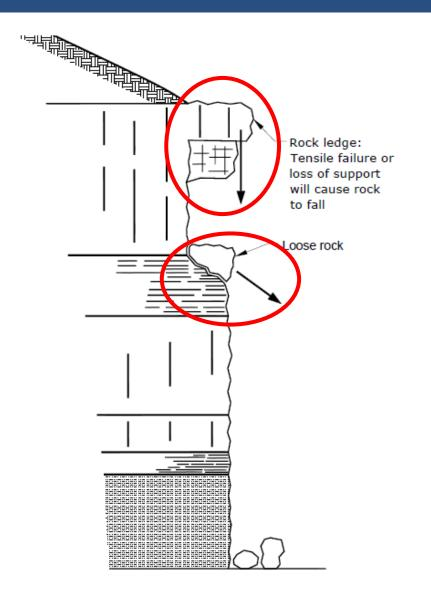
Intact blocks of rock on a fractured highwall are susceptible to falling when they are unconfined.
