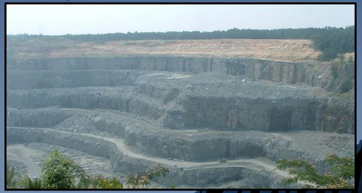
Ground control (GC) hazards are created when workers are exposed to highwalls, pit walls, banks, or slopes with the potential for failure.
