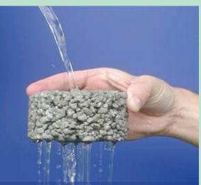
Water flows uninhibited through Portland Cement Concrete Porous Pavement.
